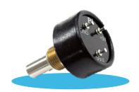
Designed to operate reliably in demanding conditions, the MagnePot 8150 series are available in three, five, and ten turn models. Incorporating Hall effect non-contacting technology means they do not wear out, as in contacting devices, and there is no degradation of the output signal over life, making them ideal for applications where minimal maintenance is required.
